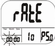
Fig. 19: Setting the sampling rate (hours)
