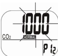
Fig. 9: Setting the CO<sub>2</sub> upper limit of NORMAL level
